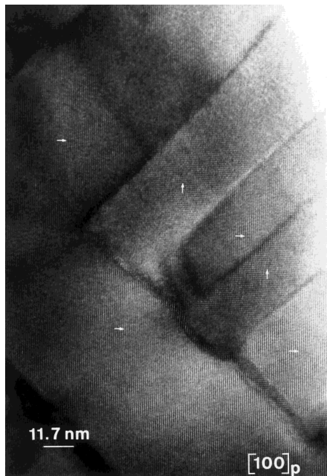
FIG. 9. \langle 100 \rangle low resolution image for a typical crystal from the composition x = 0.08 showing larger 90^\circ oriented domains which give a SAED pattern such as Fig. 7 (white arrows mark [001] directions).
